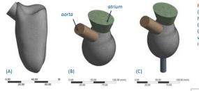
Fig. 2 Meshed geometries (tetrahedral elements) of healthy patient-specific LV (A), paradigmatic dilated LV (B), paradigmatic dilated LV with inflow cannula inserted in the apex (C)
