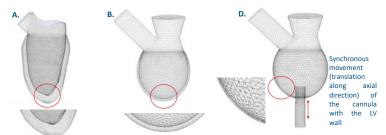
Fig. 6 End-diastolic and end-systolic meshes superimposition for the heathy LV (A), HF-LV with EF=50% (B), HF-LV with EF=10% with cannula (D). Zoom to underline the different amounts of displacement.
